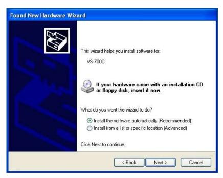
**IMPORTANT**: If the Wizard displays "UM-1" instead of "VS-700C", go back to step 1 and make sure your DIP switches are setup properly.
