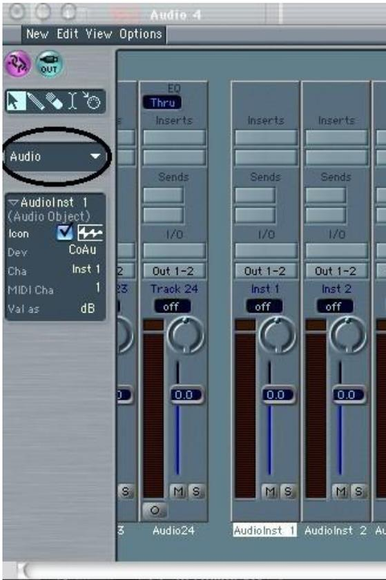
Clicking on the topmost of the two I/O bars in an instrument strip gives you a popup where you can pick an instrument.
