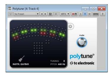
The display above is indicating that the E, G, and B strings are slightly flat, with the G string being most out of tune. When you start to tune an individual string, Polytune goes automatically into Chromatic mode.
