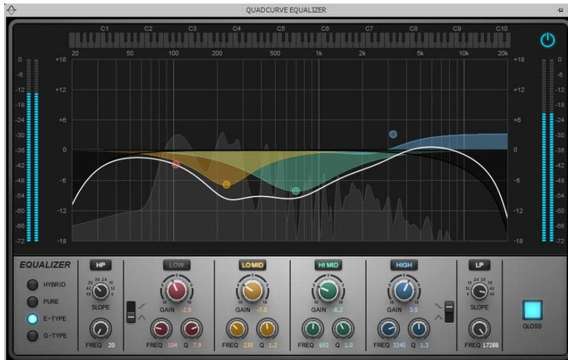
This shows the Rhythm Natural preset for the J-200. The main object is to lower two resonances from the piezo pickup, while retaining the low end and giving a slight boost in the 5 – 10 kHz range, but rolling off gently above 10 kHz to reduce some of the unnaturally high frequencies contributed by typical piezo pickups. The preset results in a natural guitar sound, like what you
