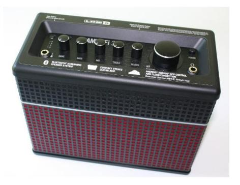
The main control panel has what you'd expect: controls for Drive, Bass, Mid, Treble, Reverb, and Output level (the latter is ringed with red LEDs so it looks cool). There's a guitar input and headphone output. Note the "Tone" button: it might seem you get only four tones, and that's
