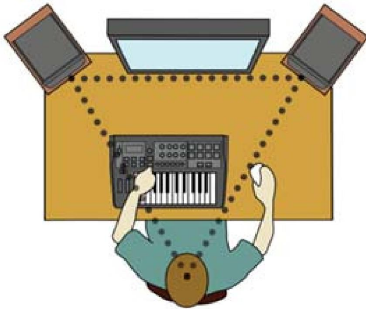
Fig. 3: When using near field monitors, the speakers should point toward the ears and be at ear level (image courtesy KRK Systems).
